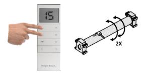
Press the LEFT UP and LEFT STOP buttons until the motor jogs twice.
