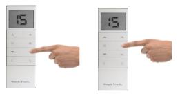
Press the RIGHT DOWN button to move the middle rail down. Click the RIGHT STOP button when you reach the bottom rail.
