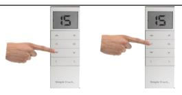
Press the LEFT DOWN button to move the bottom rail down. Click the LEFT STOP button when you reach ordered drop height.
