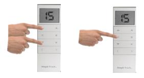
Press the DOWN and UP buttons to move the middle and bottom rails together until it reaches the headrail. Press the STOP button.
