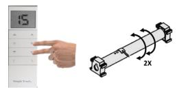
Press the RIGHT DOWN and RIGHT STOP butt until the motor jogs twice.
